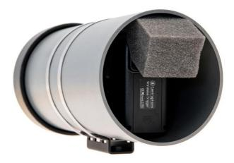
Step 5a (wireless connection): To secure the flash inside the Flash Housing Tube, lodge the Foam Wedge lengthwise on top of the receiver. Leave a portion of the Foam Wedge overhanging, as this will also help to prevent the flash being able to shift backwards once the Rear End Seal + Back Plate is applied.
